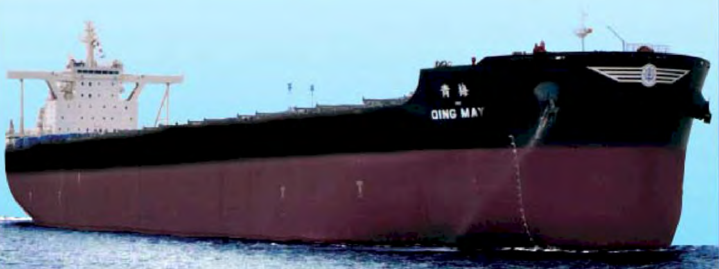
M/V "Qing May" Built April 28, 2012 Foremost's Third Vessel of Its Newly Designed 206,000 DWT "Newcastlemax" Series
